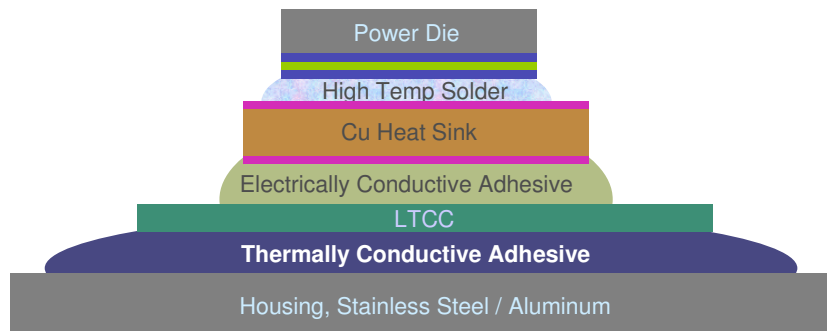
A power device where thermally conductive adhesive and electrical adhesives are applied
